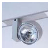
Stanley-F5 Spotlight Unit: QR111, G53, max. 1x60W LL5-YF5-L250 (L: 250mm)
